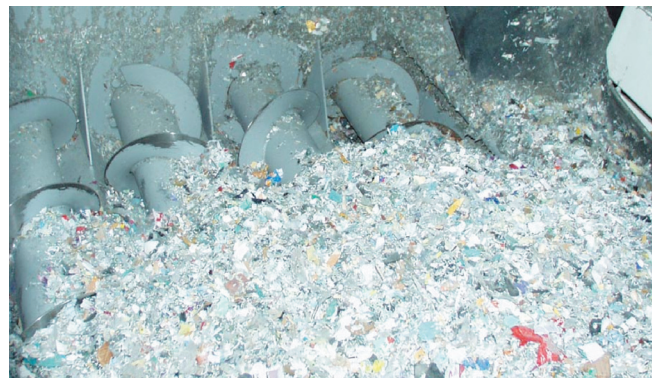
Bild 4: Screw extractor floor in the docking station Figure 4: Schneckenboden in der Andockstation
