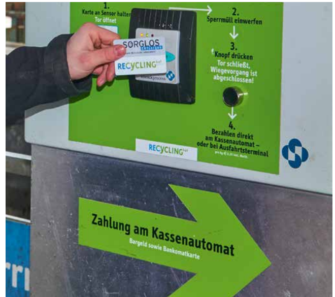
Photo 4: Waste for which a charge is payable is unloaded onto the container scales and automatically weighed. The charge is calculated on the single-use or regular-use card.
