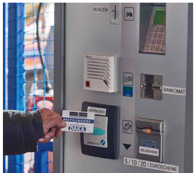
Photo 7: The customer can pay by cash or with the ID card. The machine accepts coins and notes. Change is given in three different coins and a payment receipt is printed out at the same time.
