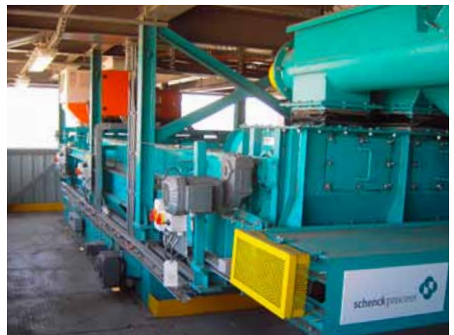
Figure 3: Belt conveyor, scanner and MULTIDOS® weighfeeder.
