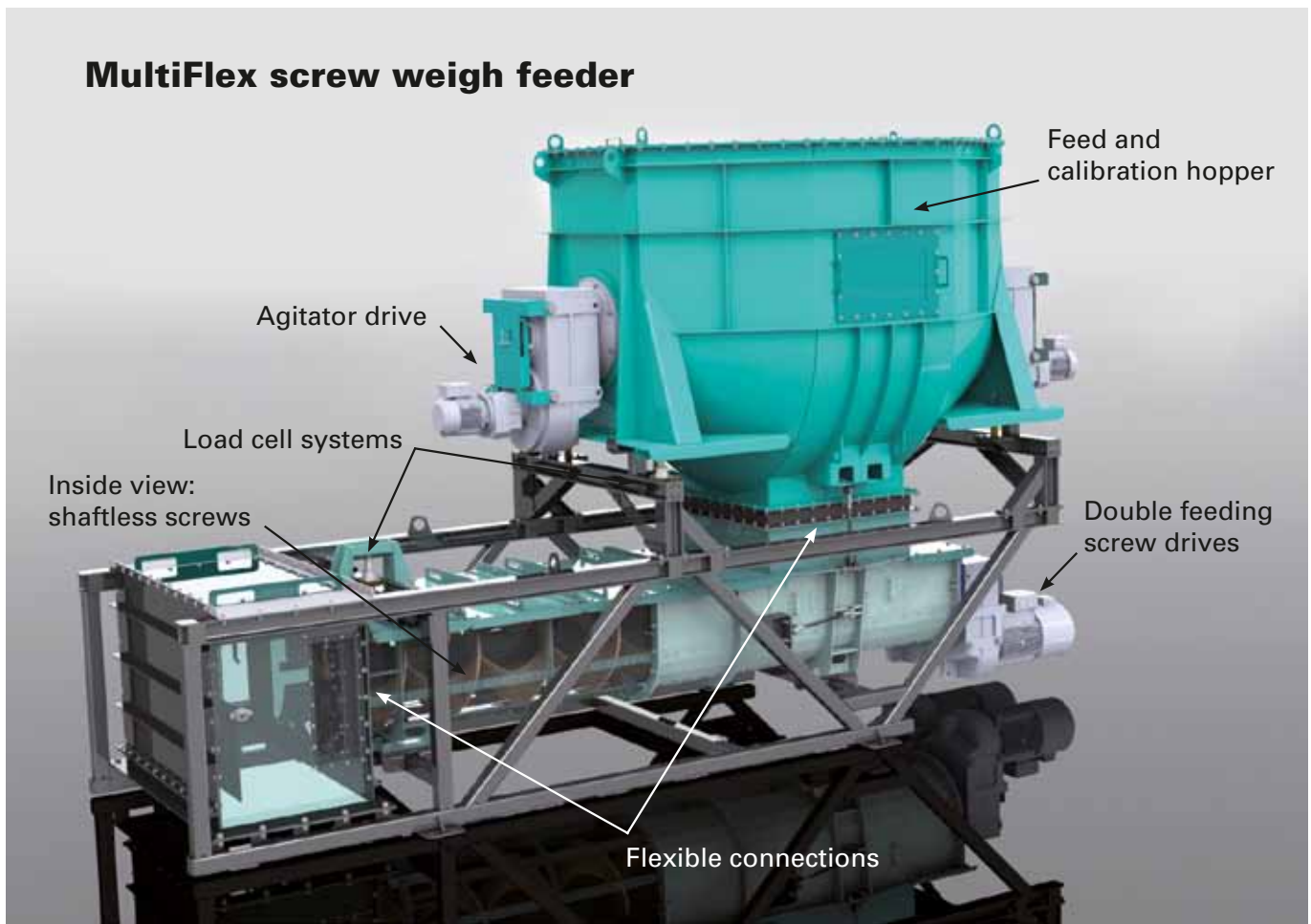
Figure 4: MultiFlex screw weighfeeder. Innovative solution for feeding alternative fuels: dust tight, double screw for pulsation free discharge, feeding and calibration hopper for on-stream calibration.
